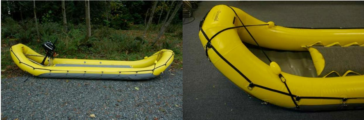
The Tow Shield installation will be easier if the RDC if it is not fully inflated.
