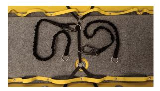
4 The two floating SS rings on the middle connecting strap are the anchors for the 6 foot long PFD tether straps.
