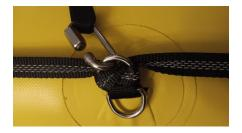
2 Attach 1/4" SS quick links to the two central grab line D rings on each side of the RDC.
