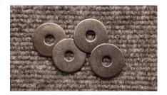
1 Replace the top and bottom washers of the center floor bolt on both sides of the RDC with the larger SS fender washers [4] using a phillips screwdriver and a 7/16" socket wrench.
