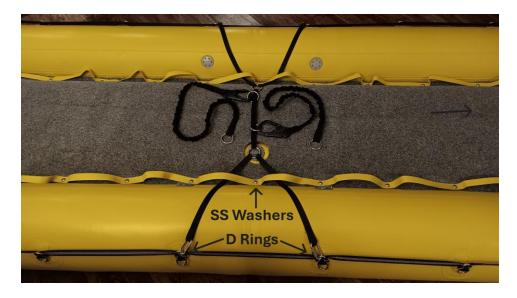
The PTA system provides secure inboard SS ring anchor points specifically designed for PFD safety tether attachments. With the extendable 6 foot long tether, responders can easily access both ends of the RDC.
