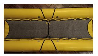
3 Starting from the center of the floor, pass each of the four PTA strap ends under the yellow hand loops and connect them to the SS quick links. Tighten securely.
